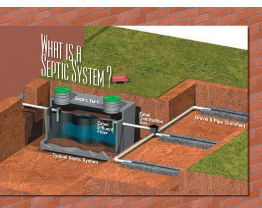
Septic systems are individual wastewater treatment systems that collect, treat and dispose of wastewater. They are reliable, cost effective and efficient. Septic systems are used were municipal sewers are not available or are impractical.
